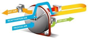
The STAD system uses two independent air flows. The main air flow will be dried, the secondary air flow of lesser volume will be used to evacuate the moisture retained by the desiccant rotor.
